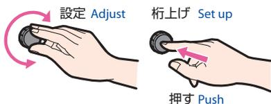
The jog dial is used for output current and voltage setup. One dial is capable of digit-by-digit numerical value setup and moving through values, which allows easy setup.
